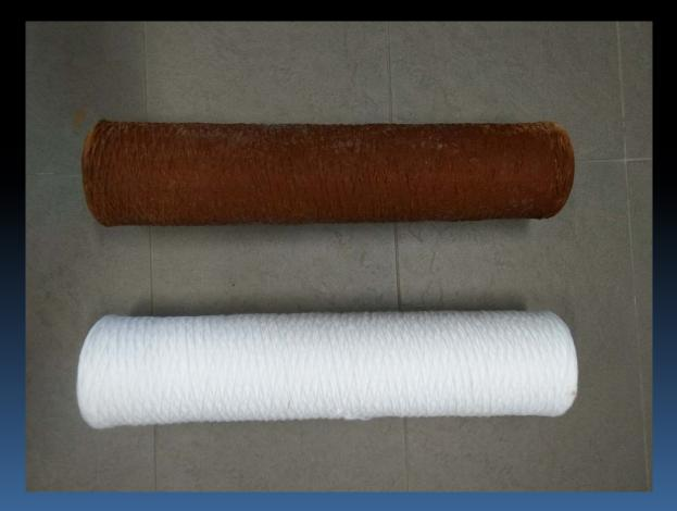
Filter cartridge from the Ritchie well after 3 hours of operation compared to a new cartridge
